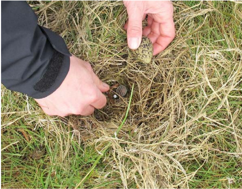
Figure 6. Installing an iButton in a nest. The nail was pushed in the ground so that it would not damage the egg, and the temperature sensor was covered with a thin layer of grass to disguise the iButton and cushion the eggs, which were then replaced in the nest. (Photo: Maggie Grenham)
