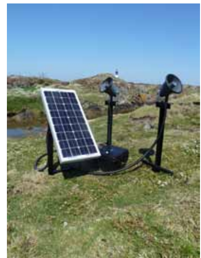
Figure 1 Spark 4 custom made solar powered sound system
