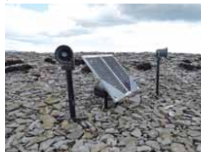
Figure 4 Solar-powered acoustic attractant system
