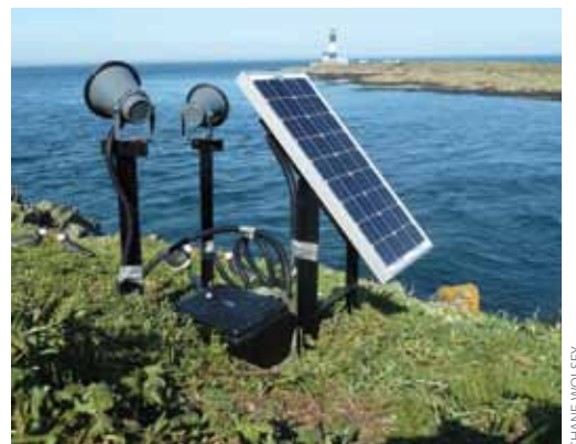
Figure 2 Solar power sound system deployed on Lighthouse Island (overlooking Mew Island) to attract Puffins
